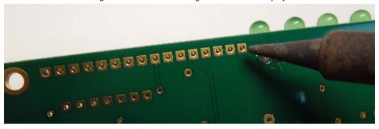
Figure 14 - Solder remaining connections on K44 board
