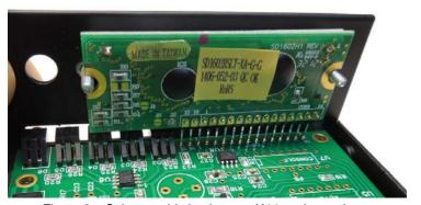
Figure 8 – Subassembly in place on K44 enclosure base
