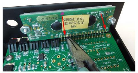
Figure 11 – Gently adjust header for equal pin alignment
