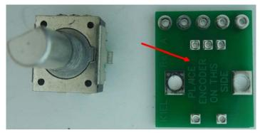
Figure 16 - Encoder and encoder PCB
