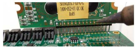
Figure 13 - Solder remaining connections on display
