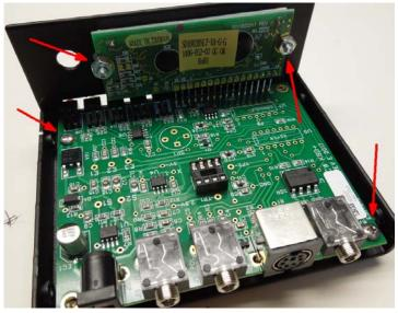
Figure 9 – Add 4-40 nuts and screws to hold subassembly in place
