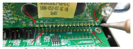
Figure 12 – Solder four places to fix display alignment
