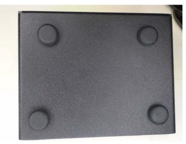
Figure 4 - Rubber feet in place on bottom half of enclosure
