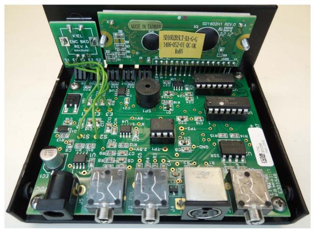
Figure 21 - Rear view with encoder and display in place
