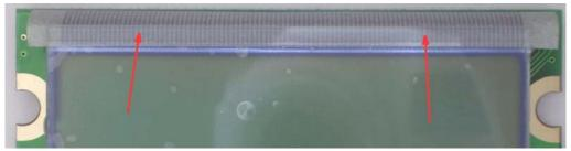
Figure 3 - Caution, do not damage ribbon film interconnect
