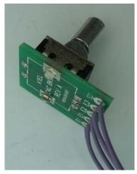
Figure 18 - Encoder on encoder PCB
