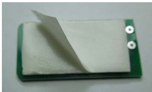
Figure 6 – Remove foam tape paper film
