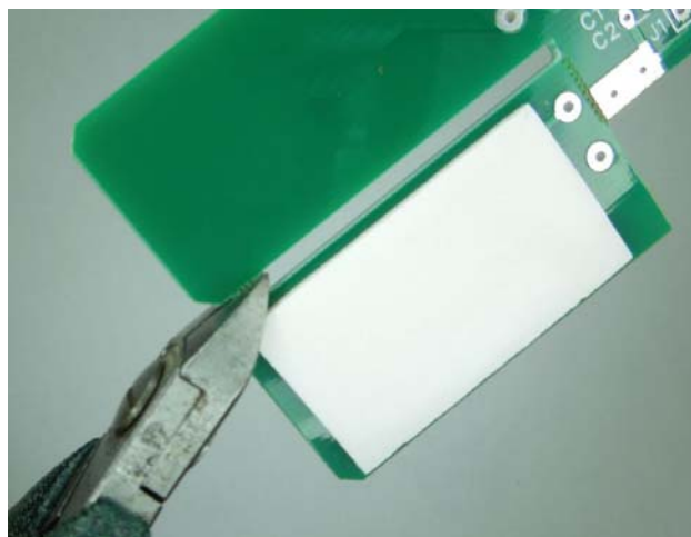
Figure 3 – Cut paddle separator
