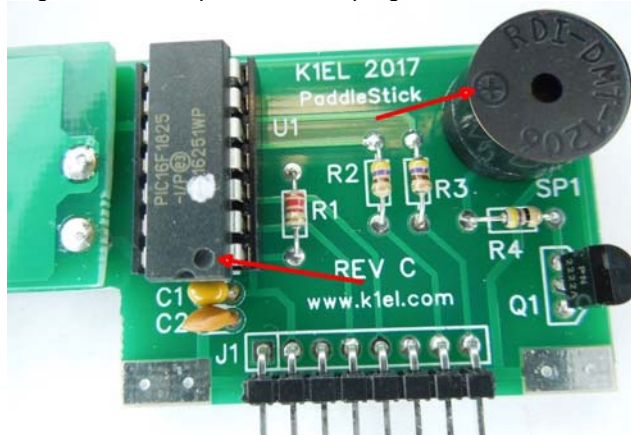
Figure 14 – Straighten leads on U1, then install speaker, transistor Q1, and U1.
