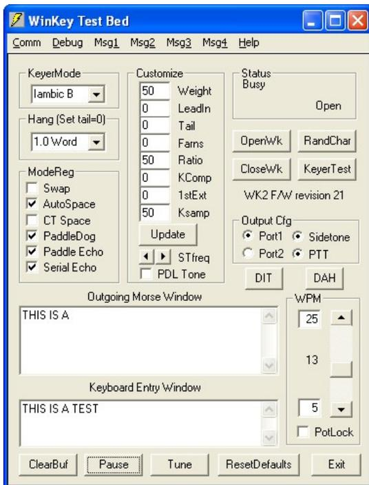
You can type into the Keyboard Entry Window and you should see the Busy status indicator turn on and off. Since WK2 Serial does not have a sidetone output you will not hear anything until you connect it to your transceiver. If serial echo is on then what you type will be echoed in the Outgoing Morse Window.
