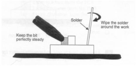
Fig. C2 - Spread solder around the work
