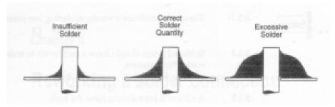
Fig. C4 - Solder quantity comparison
