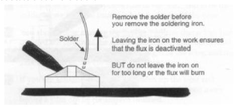
Fig C3 - Remove the solder
