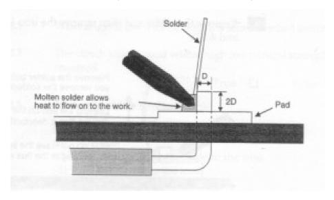
Fig. C1 - Form a heat bridge
