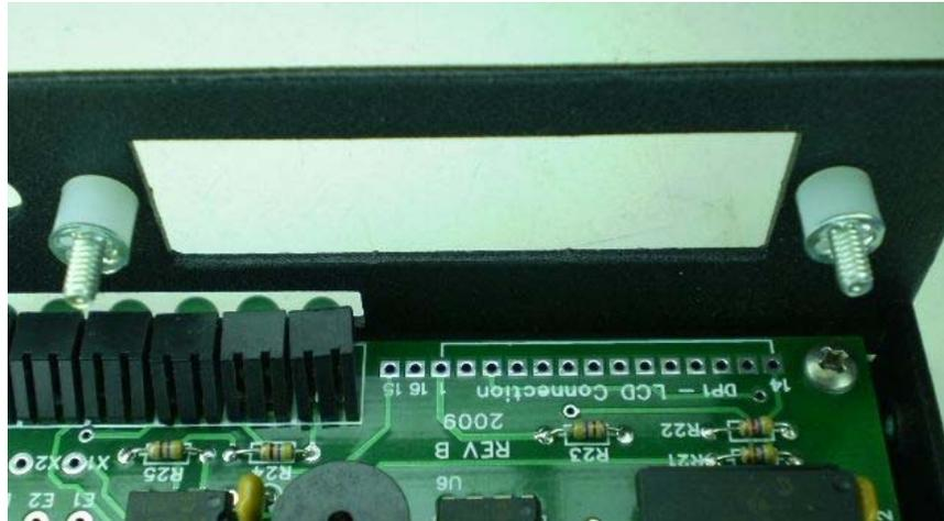
Now carefully install the display so that the header pins fit into the K42 board and the LCD mounting ears fit in place on the threaded studs. This will take a little coaxing to get into place. Please remember to handle the display on its sides so as not to damage the display's wire film ribbon cable (looks like paper).
