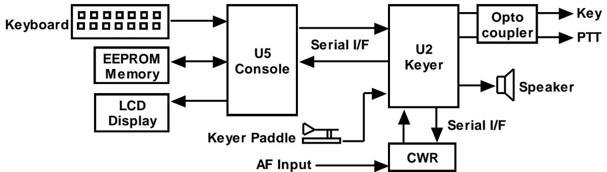
Figure 6 - K42 CW Keyboard Block Diagram
